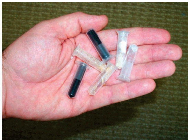
Figure 2. Stockpiled microcentrifuge tubes containing 50 mg of a variety of different adsorbents facilitate adsorbent screening studies.
